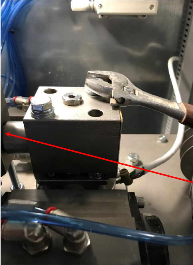
Remove block. Prise off block from cyclone side. Remove valve V002
