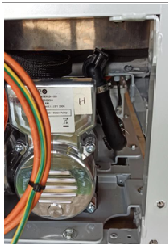
Fig. 7 eBTM 2.0 fluid purging valve at the outlet of the radiator
